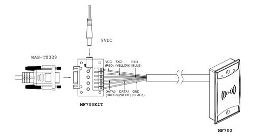
Note: MF700KIT is a test connection kit for MF700 configuration use. It is an optional item for purchasing.
