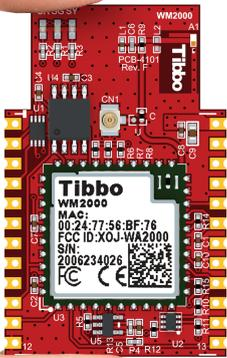
The WM2000 is the latest programmable wireless Industrial IoT (IIoT) module offered by Tibbo. It implements Wi-Fi and Bluetooth Low Energy (BLE) interfaces that introduce several new features, such as wireless debugging, over-the-air (OTA) updates, and TLS support.
