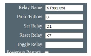
Enter D1 in relay 22 Set Relay box and, as the relay will be reset by the sequencer, enter K7 in the Reset Relay box. Also enter K8 and K9 into relay 23 and relay 27 pulse/follow boxes. While we are in the relay section, lets rename the relays to better reflect their functionality.
