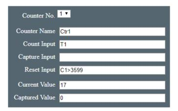
Using T1 for the count input will make the counter increment once per second. There are 3600 seconds in 1 hour so we reset the counter when its greater than 3599 with C1>3599. The counter will count from 0-3599.
