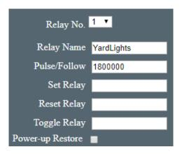
The above example will turn off the yard lights after 30 minutes. 1800000 mS is 1800 seconds. 1800 seconds is 30 minutes.
