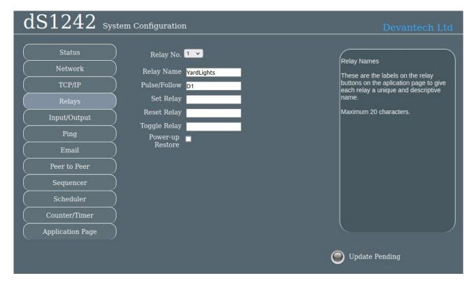
Use the Relay No. box to select the relay to configure. There are 32 relays available. Relays 1 & 2 are the physical relays on the module. Relays 3-32 are virtual relays, they have no physical presence but otherwise behave the same as the real ones. I/O lines may be linked to virtual relays to provide additional physical outputs, see next section for details.
