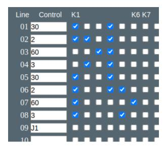
Here we hold both lights at Red for 30 seconds to give traffic time to traverse the controlled area. Then Red + Amber for two seconds followed by Green for 60 seconds. We then stop the traffic with Amber for 3 seconds followed by Red. Again we hold both lights at Red for 30 seconds before letting the other queue through at line 6.
