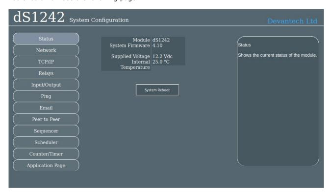
This status page shows you the system firmware revision as well as the supplied voltage to the board and its internal temperature.
