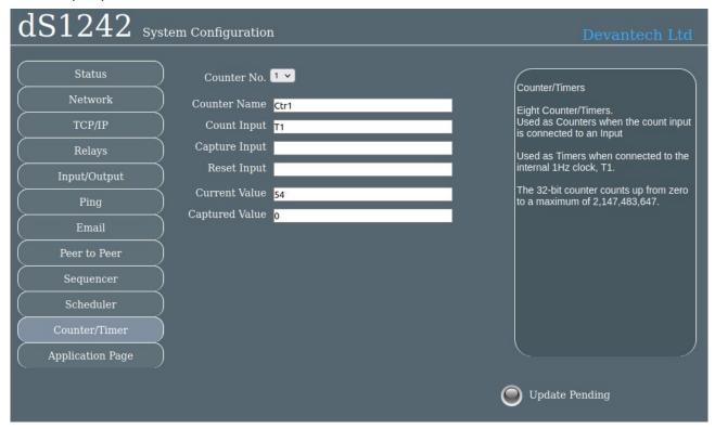
There are a total of eight counter/timers available, selected with Counter No. box. Each counter can count at a maximum speed of 20Hz (20 counts per second).
