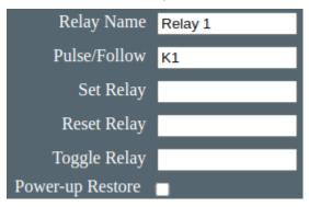
Placing K1 in a relays Pulse/Follow box will make the relay follow the K1 output, in this case pulsing the relay on and off every two seconds.
