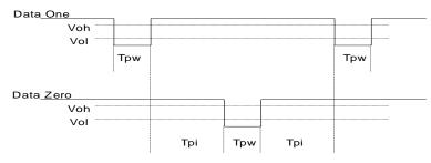
Tpw Pulse Width Time -- 20  $\!\mu\text{Sec}$  (minimum) to 100  $\!\mu\text{Sec}$  (maximum)
