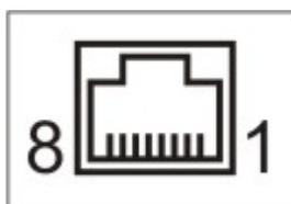
Ethernet port of the DS100 is of 10BaseT type. The DS100 is compatible with all 10BaseT Ethernet hubs and also 99% of 100BaseT hubs. This is because most 100BaseT hubs are actually 100/10 devices that auto-detect the type of device connected to each port.
